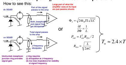
Single SQUID at 4.2K:  $T_n$ ~10K room-temp amplifier doable but difficult **SQUID** array at 4.2K: same  $T_n$  as single SQUID, just different  $R_n$ Single SQUID at 0.4K: T<sub>n</sub>~1K room-temp amplifier very difficult Single SQUID read with single SQUID: 2nd SQUID limits dynamic range Single SQUID read with a k-SQUID array:
